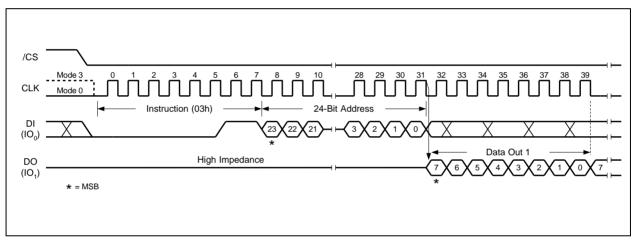
Figure 14. Read Data Instruction 32-Bit Address is required when the device is operating in 4-Byte Address Mode
