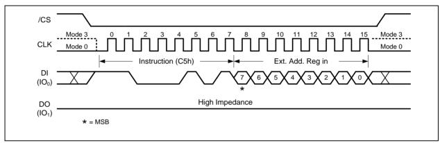
Figure 11. Write Extended Address Register Instruction
