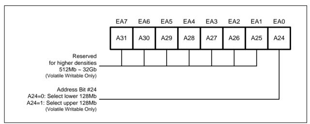
Figure 3e. Extended Address Register (Single Die W25Q256JW-IQ)
