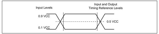
Figure 59. AC Measurement I/O Waveform
