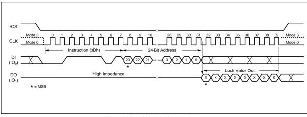
Figure 54. Read Block Lock Instruction 32-Bit Address is required when the device is operating in 4-Byte Address Mode
