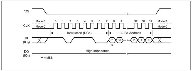
Figure 38. 64KB Block Erase with 4-Byte Address Instruction
