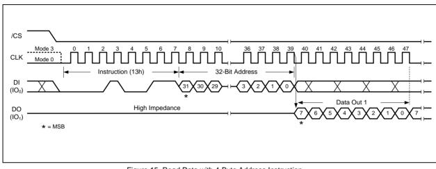
Figure 15. Read Data with 4-Byte Address Instruction
