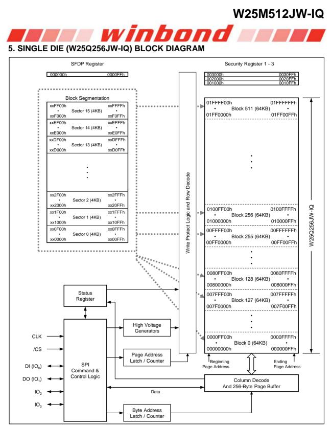
Figure 2b. Single Die W25Q256JW-IQ Serial Flash Memory Block Diagram
