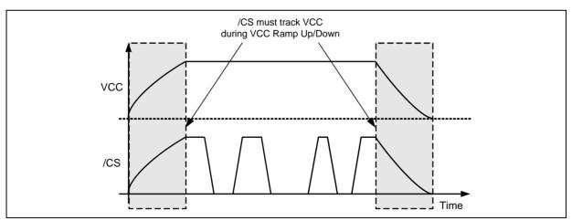
Figure 58b. Power-up, Power-Down Requirement
