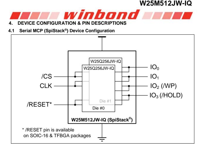
Figure 2a. W25M512JW-IQ Device Configuration
