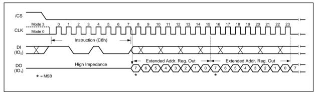
Figure 10. Read Extended Address Register Instruction
