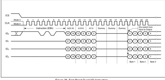
Figure 26. Fast Read Quad I/O Instruction 32-Bit Address is required when the device is operating in 4-Byte Address Mode
